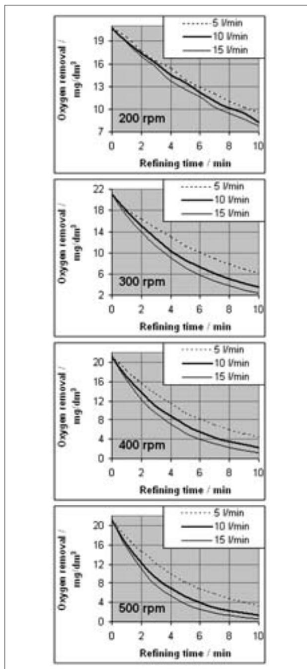
Figure 6 Results of oxygen removal from water in URO-200 reactor
