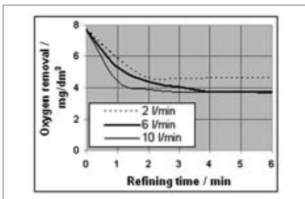
**Figure 7** Results of oxygen removal from water in URC-7000 reactor
