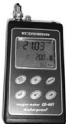
Figure 5 Oxygen meter Elmetron CO-401
