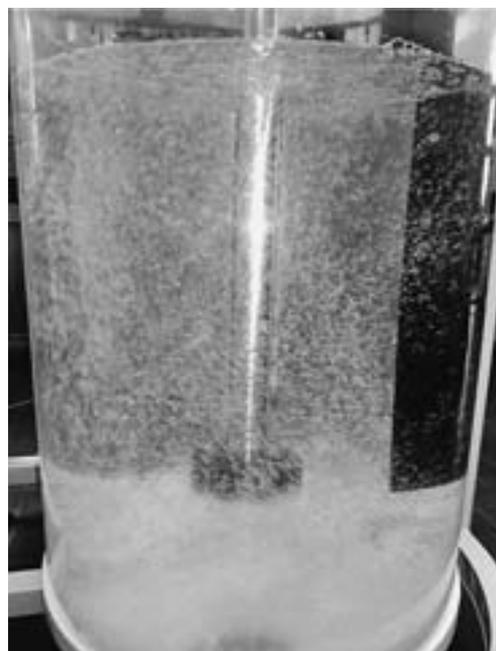
**Figure 8** Uniform dispersion of refining gas in the liquid metal (400 rpm, 10 dm<sup>3</sup>/min)
