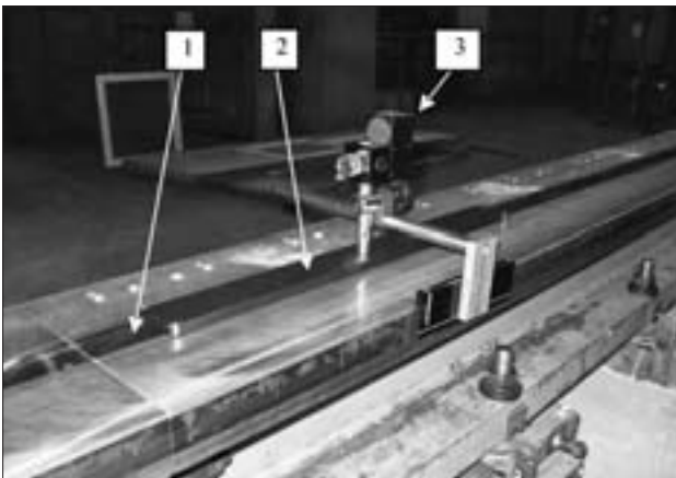
Figure 5 View of the measuring set: 1 – investigated surface (location of the carriage), 2 – prepared 500 mm foot, 3 – measuring optical set
