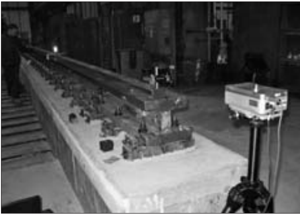
Figure 4 Setting the straightness of the slide top surface
