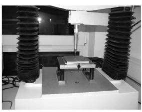
Fig. 3. Indentation testing of the rat femur.
