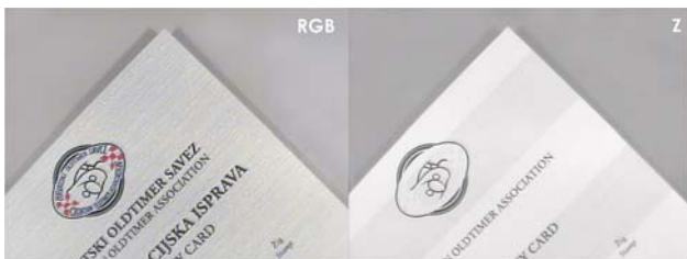
Figure 8 Photos of IRD-protected driver's license with the ZRGB device: RGB image (visible text and logo) and Z image (part of the text and the logo is gone)
