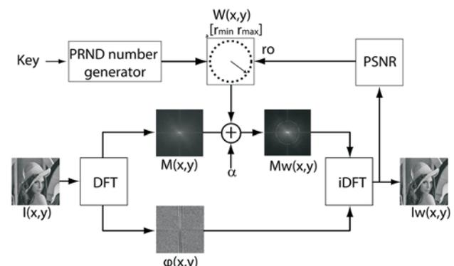
Figure 2 Block diagram of the encoder
