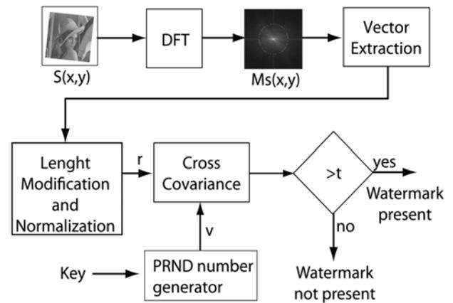
Figure 4 Block diagram of the decoder
