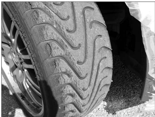
Figure 14 Wear of the used tire after 45 min of driving Slika 14. Istrošenje korištene gume nakon 45 min vožnje
