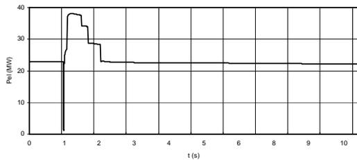
Figure 6. Electrical power production response of units G3 and G4, an islanding scenario with consumption surplus
