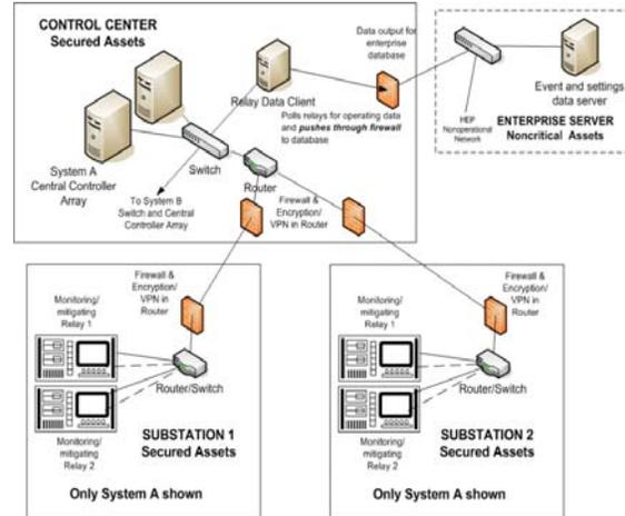
Figure 10. Secure communications architecture
