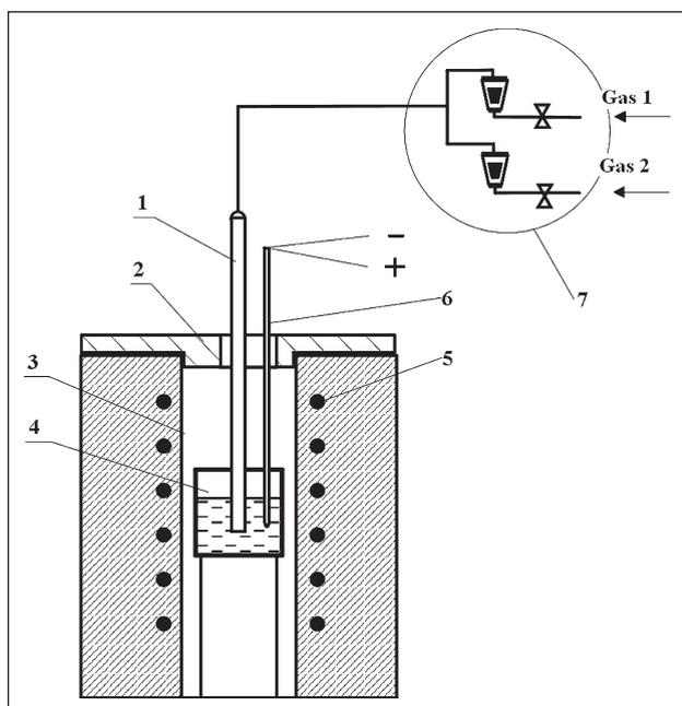
**Figure 1** Sketch of equipment used in tests: 1 - lance, 2 - asbestos seal, 3 - ceramic shield, 4 - crucible with alloy, 5 - furnace heating components, 6 - thermocouple, 7 - gas supply system.
