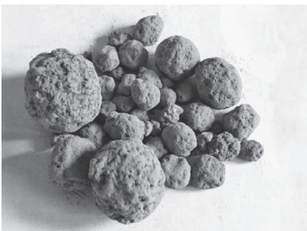
Figure 4 Pellets prepared from the dust from cold blast cupola furnace
