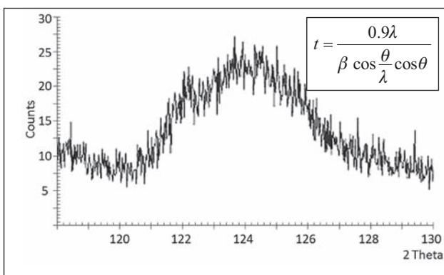
Figure 5 XRD diffraction peak of TiN(422)
