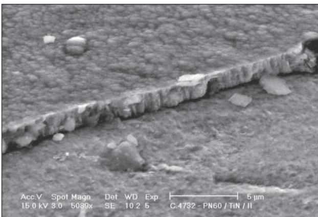
Figure 6 Surface morphologies of TiN(PVD) implanted with nitrogen
