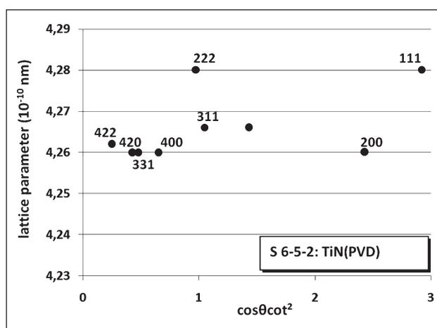
Figure 4 The Cohen-Wagner plot, lattice parameters  $a_{hkl}$  vs.  $\cos^2\theta$ .
