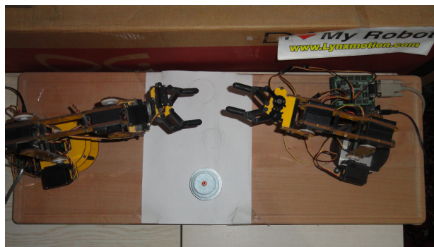
Figure 5. Experimental setup, two robotic arms and the TOH(3) disk set.
