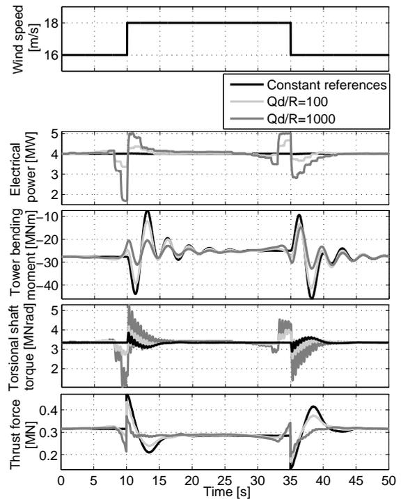
Fig. 6. Deterministic disturbance - Reducing tower loads
