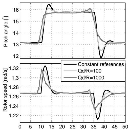
Fig. 7. Deterministic disturbance - Reducing tower loads (states)
