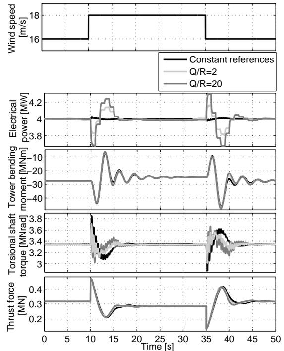
Fig. 8. Deterministic disturbance - Reducing shaft loads
