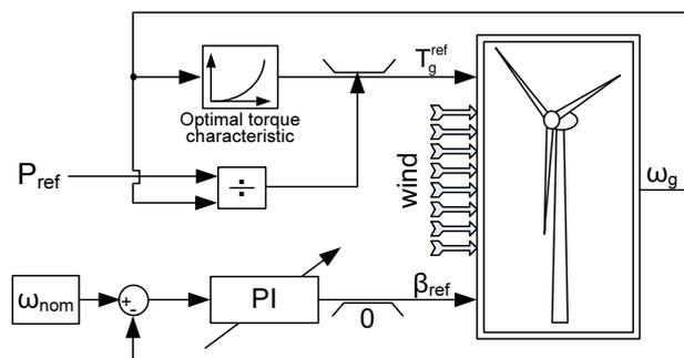
Fig. 3. Wind turbine controller operation principle
