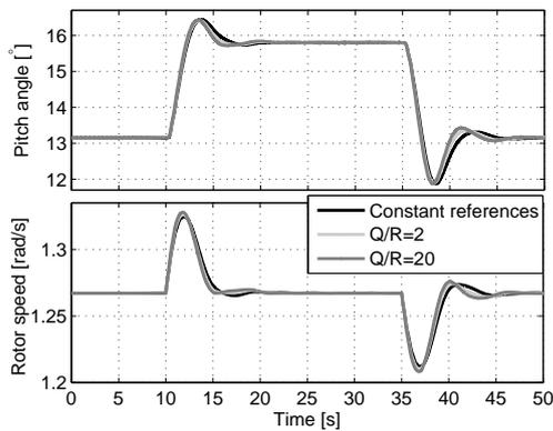
Fig. 9. Deterministic disturbance - Reducing shaft loads (states)
