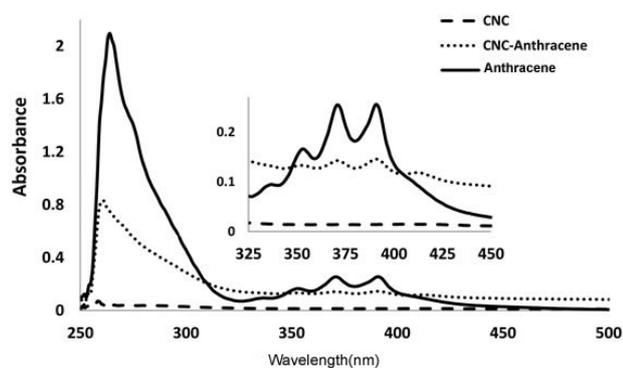
**Figure 2.** UV light absorption spectra of anthracene (solid line), CNC-Anthracene (dotted line) and CNCs (dashed line).
