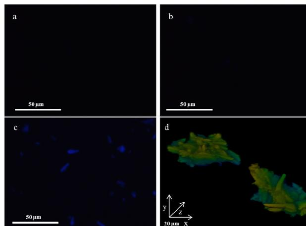
**Figure 1.** a) Fluorescence photomicrograph of TEMPO-oxidized cellulose nanocrystals. b) Fluorescence photomicrograph of the cellulose material after the reaction between TEMPO-oxidized cellulose nanocrystals and azidocoumarin (negative control). c) Fluorescence photomicrograph of CNC-Coumarin dispersed in water. d) 3D reconstructions of 45 images taken at different focus levels (CNC-Coumarin).
