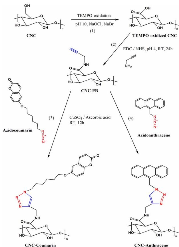
Scheme 1. Schematic representation of the synthetic route for the photoresponsive cellulose nanocrystals.
