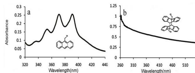
**Figure 3.** UV light absorption spectra of anthracene (a) and photodimerized anthracene (b).
