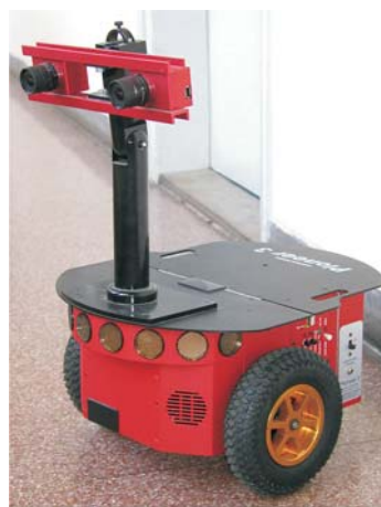
Figure 2 Mobile robot Pioneer 3DX equipped with a stereo camera system Videre design STH DCSG-STOC.
