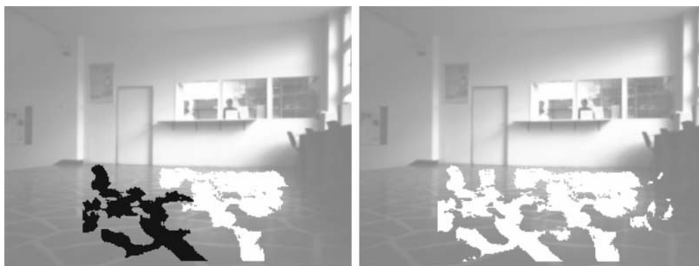
Figure 4 In the case where dilation is not applied, two surfaces are detected corresponding to the floor surface. These surfaces are represented by the black and white region in the left image. In the case where dilation is applied, these two surfaces are merged into a single floor surface represented by the white region in the right image.
