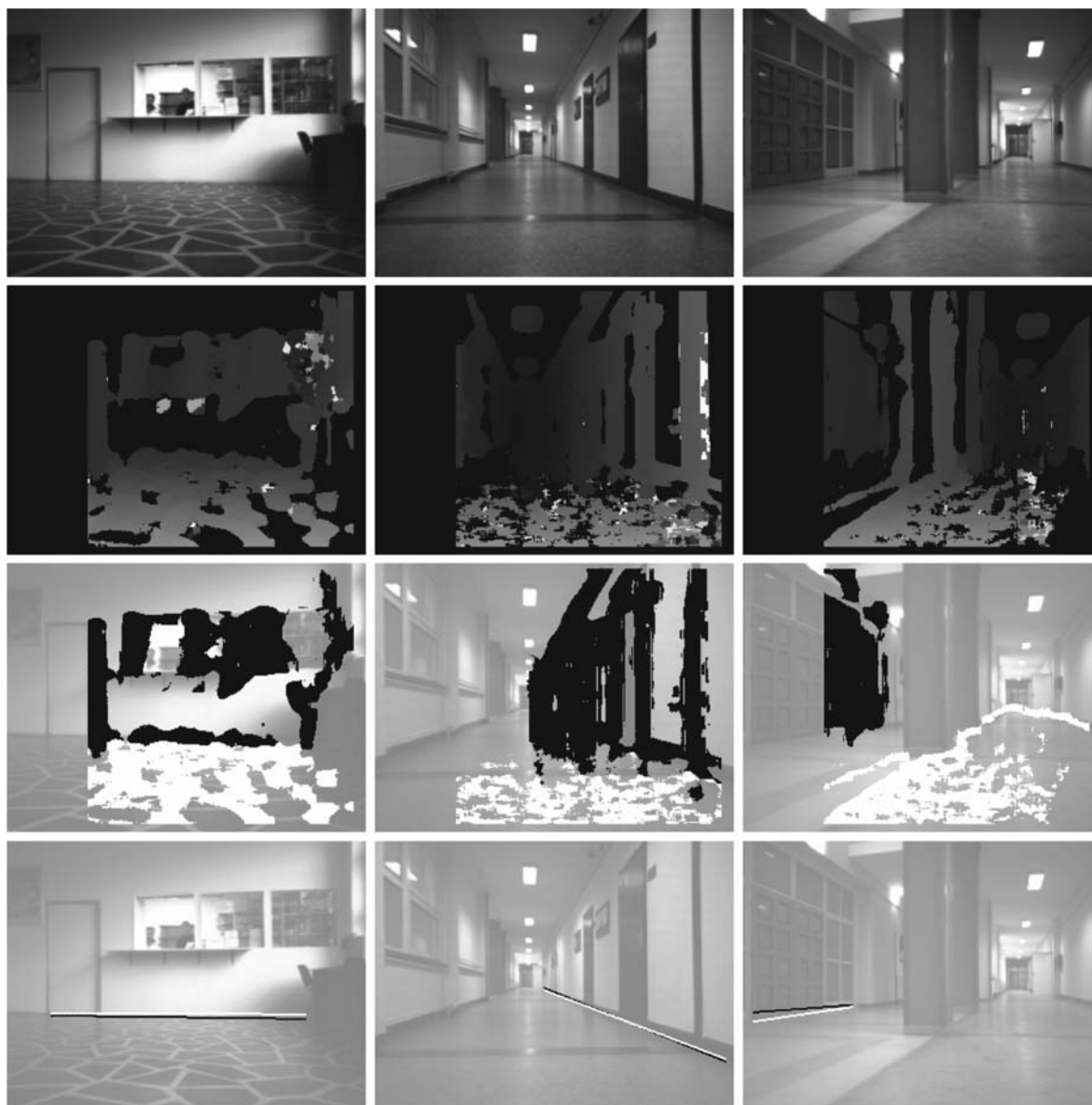
Figure 3 Images taken by the left camera mounted on a mobile robot (first row); the corresponding disparity images (second row); the result of the image segmentation (third row): detected floor surface (white) and the dominant wall surface (black) and performance index (last row): GT line (white) and the reference line (black).
