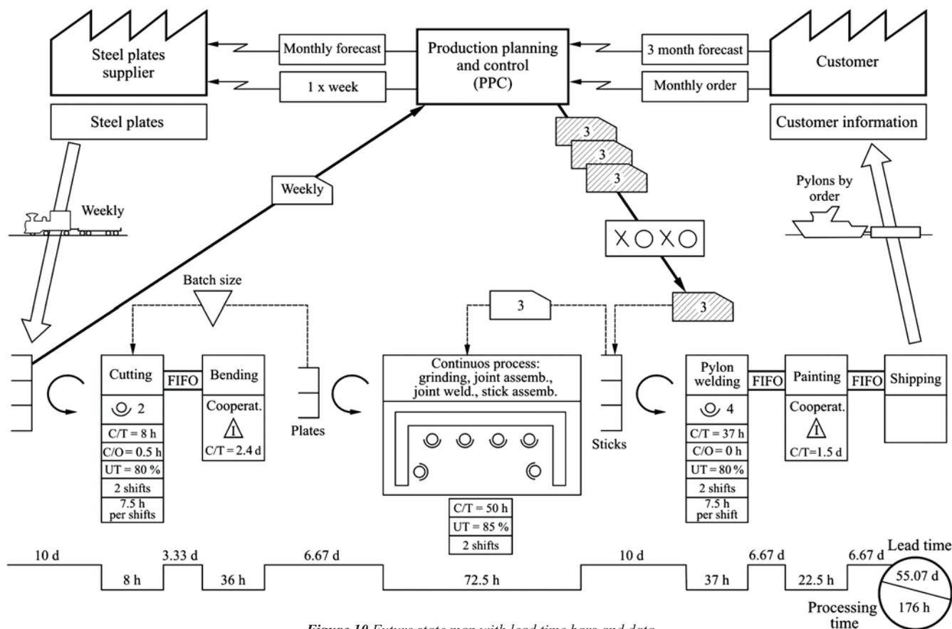
Figure 10 Future state map with lead time bars and data
