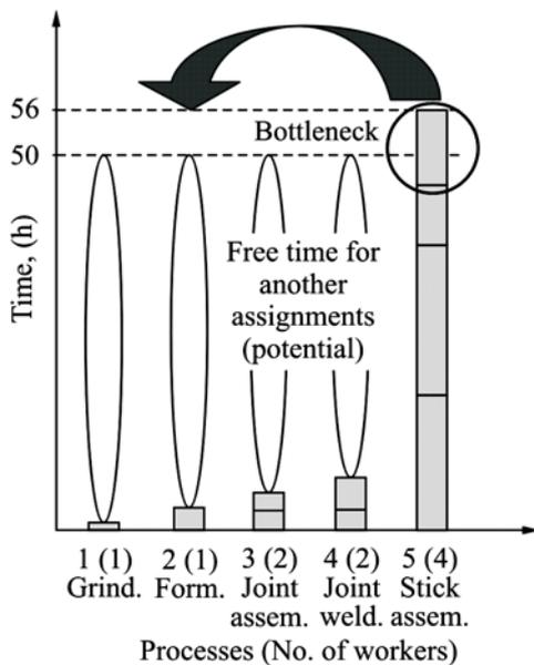
Figure 7 Current state worker assignments
