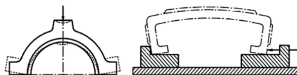
Figure 1 Deformation of a work piece during clamping Slika 1. Deformacija radnog komada kod stezanja
