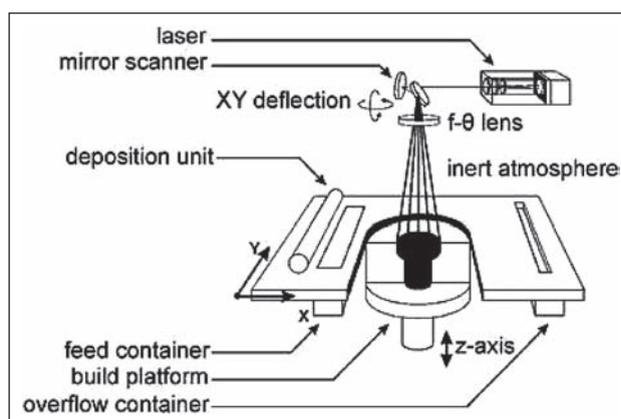
Figure 2 Principle of the SLM [18]
