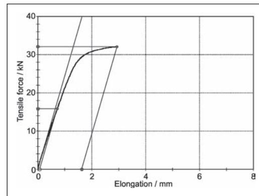
Figure 6 Tensile curve for specimen No. 2
