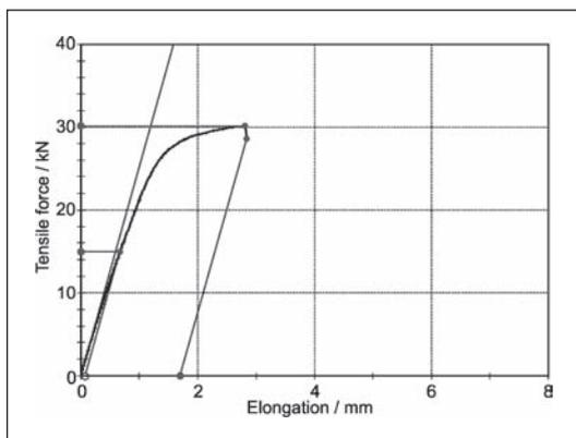
Figure 5 Tensile curve for specimen No. 1
