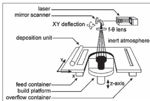
Figure 2 Principle of the SLM [18]
