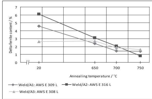
**Figure 4** Delta-ferrite transformation depending on annealing temperature during t=2 hours
