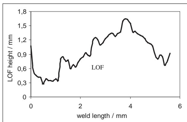
Figure 6 LOF profile between the molten pool and parent material
