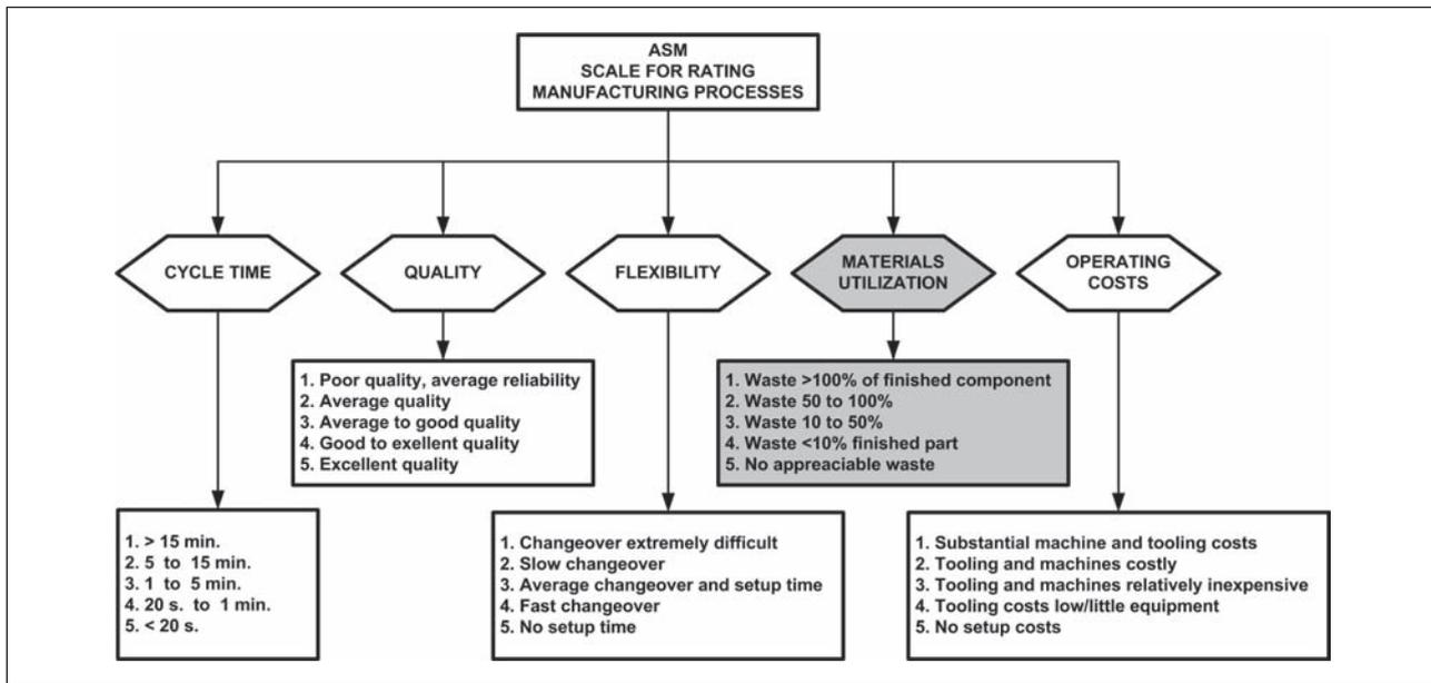
Figure 4 Parameters of manufacturing process in the metalworking industry (Rating: 1-poorest; 5-best) [9]
