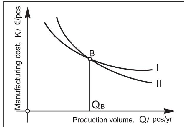
Figure 6 Diagram of the total manufacturing costs per product unit, for two blank variants [13]
