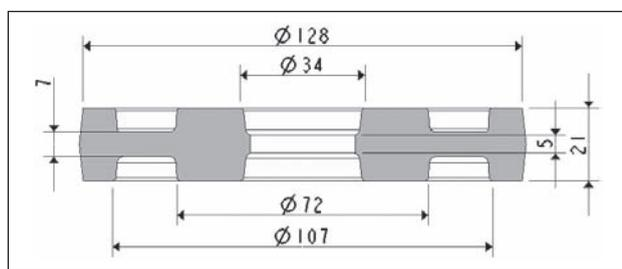
Figure 5 Group forging for the gear group from Table 1
