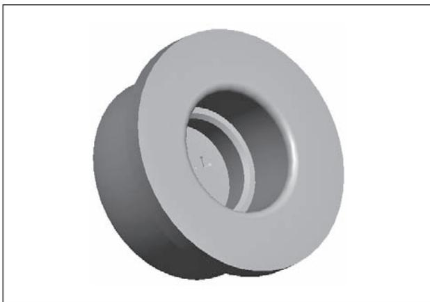
**Figure 2** Group blank manufactured by cold bulk forming
