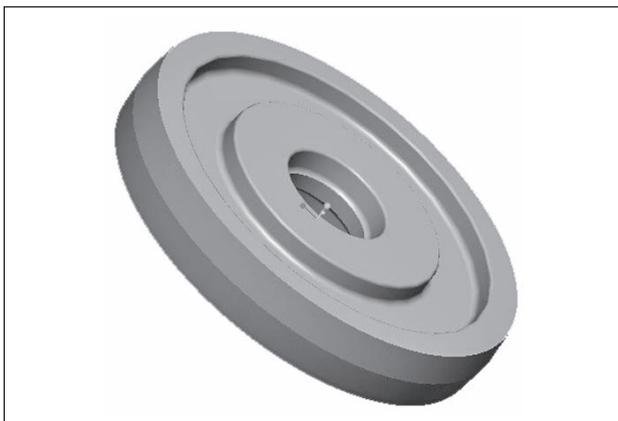
**Figure 3** Group blank manufactured by closed die forging
