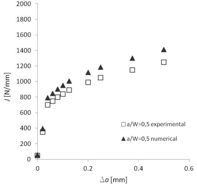
Figure 6. Verification of numerically obtained *J*-integral values on AISI 304LN
