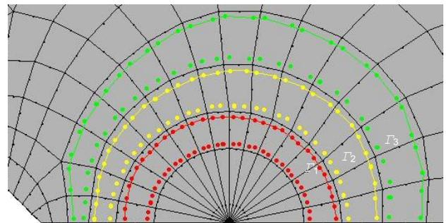
Figure 2.  $J$ -integral contour paths ( $\Gamma_1$ ,  $\Gamma_2$ ,  $\Gamma_3$ ) surrounding the crack tip through the integration points of finite elements
