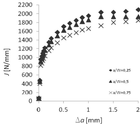
Figure 7. AISI 420: predicted *J* values for crack extension  $\Delta a$
