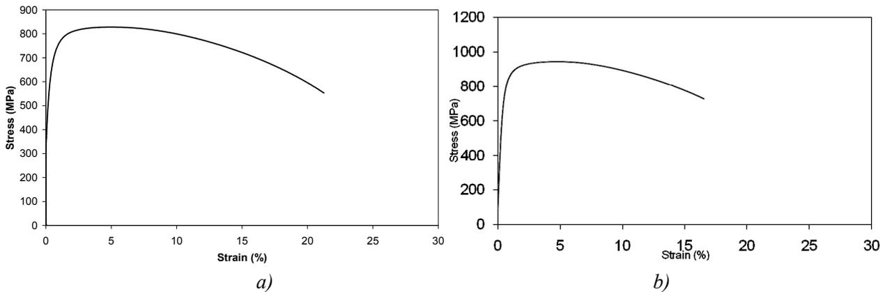
Figure 3. Stress-strain curve for: a) AISI 420. b) AISI 431.
