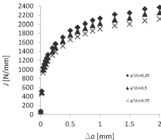
Figure 8. AISI 431: predicted  $J$  values for crack extension  $\Delta a$ .
