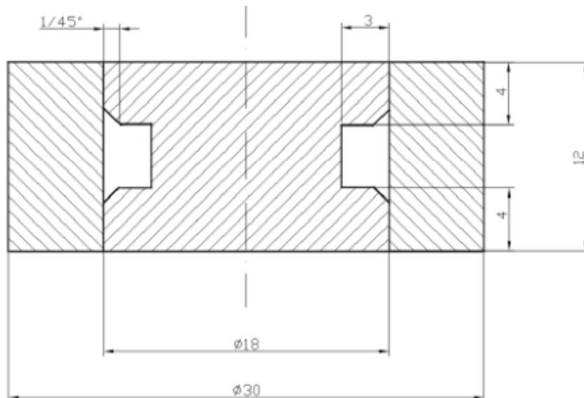
Figure 5. Dimensions of bimetallic components
