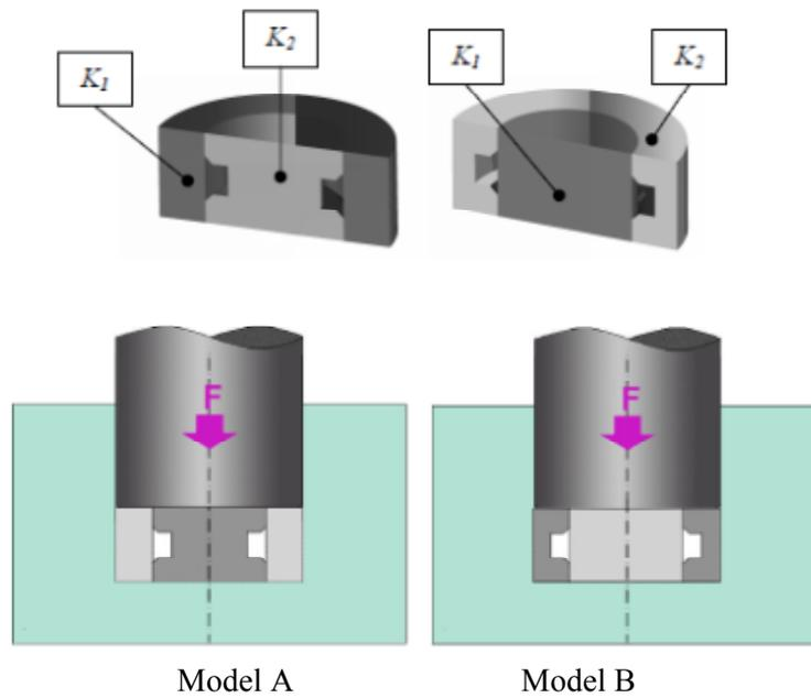
Figure 4. Two models of bimetallic joining
