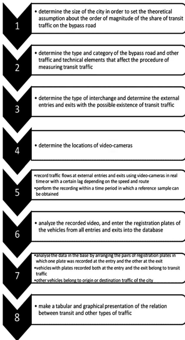
Figure 4 Model of transit traffic measuring at urban bypass roads
