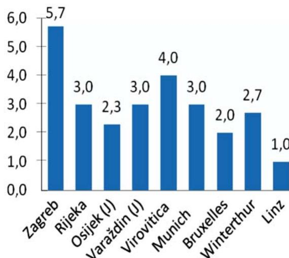
Figure 1 Average distance between the interchanges at bypasses
