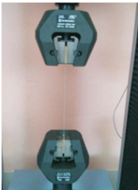
Figure 1 Testing machine and single strap sample
