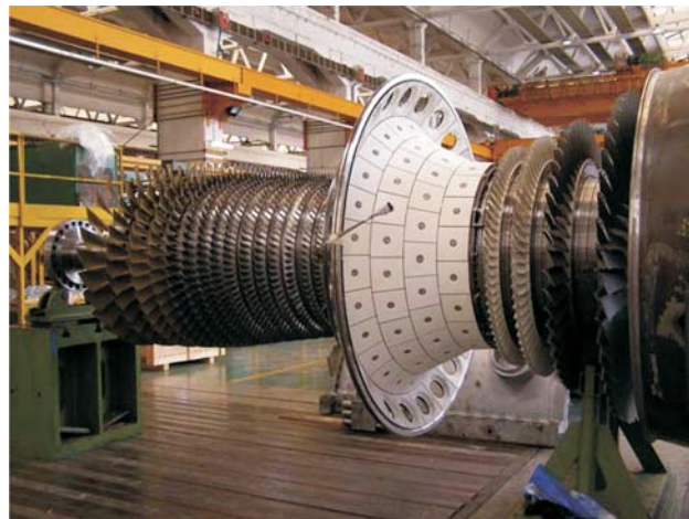
Figure 3 Rotor view with annular combustion chamber
