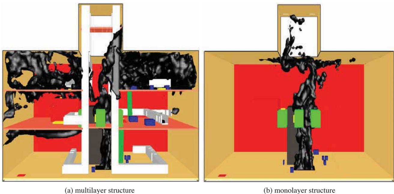
Figure 4 The  $0.0001 \text{ kg/m}^3$  equivalent distribution of the smoke concentration
