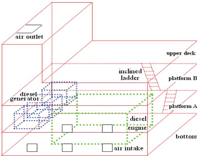
Figure 1 The structure diagram of a typical engine room
