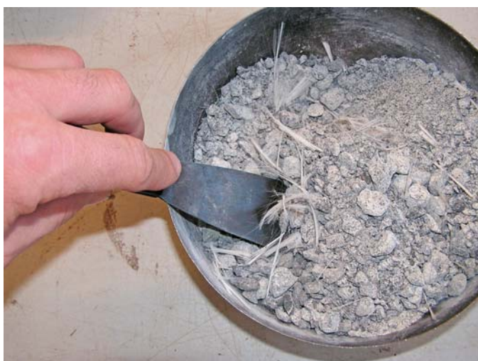
SLIKA 13 – Skupljanje vlakana u snopiće prilikom miješanja FIGURE 13 – Clustering of fibre bundles during mixing
