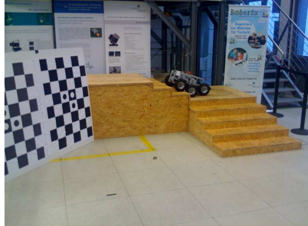
Fig. 4. The scene of the first experiment carried out in the Robotik Pavillion at Fraunhofer IAIS, Sankt Augustin. The scene consists of a wooden staircase with a robot on it, some posters and a calibration pattern. The robot moved on a square with 120 cm side length.
