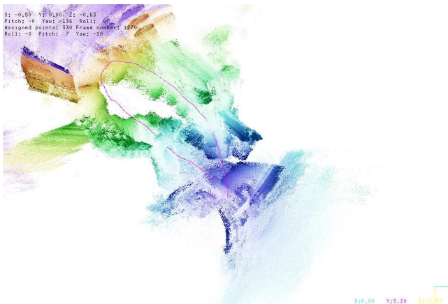
Fig. 1. The resulting 3D map based on the estimated ego-motion.
