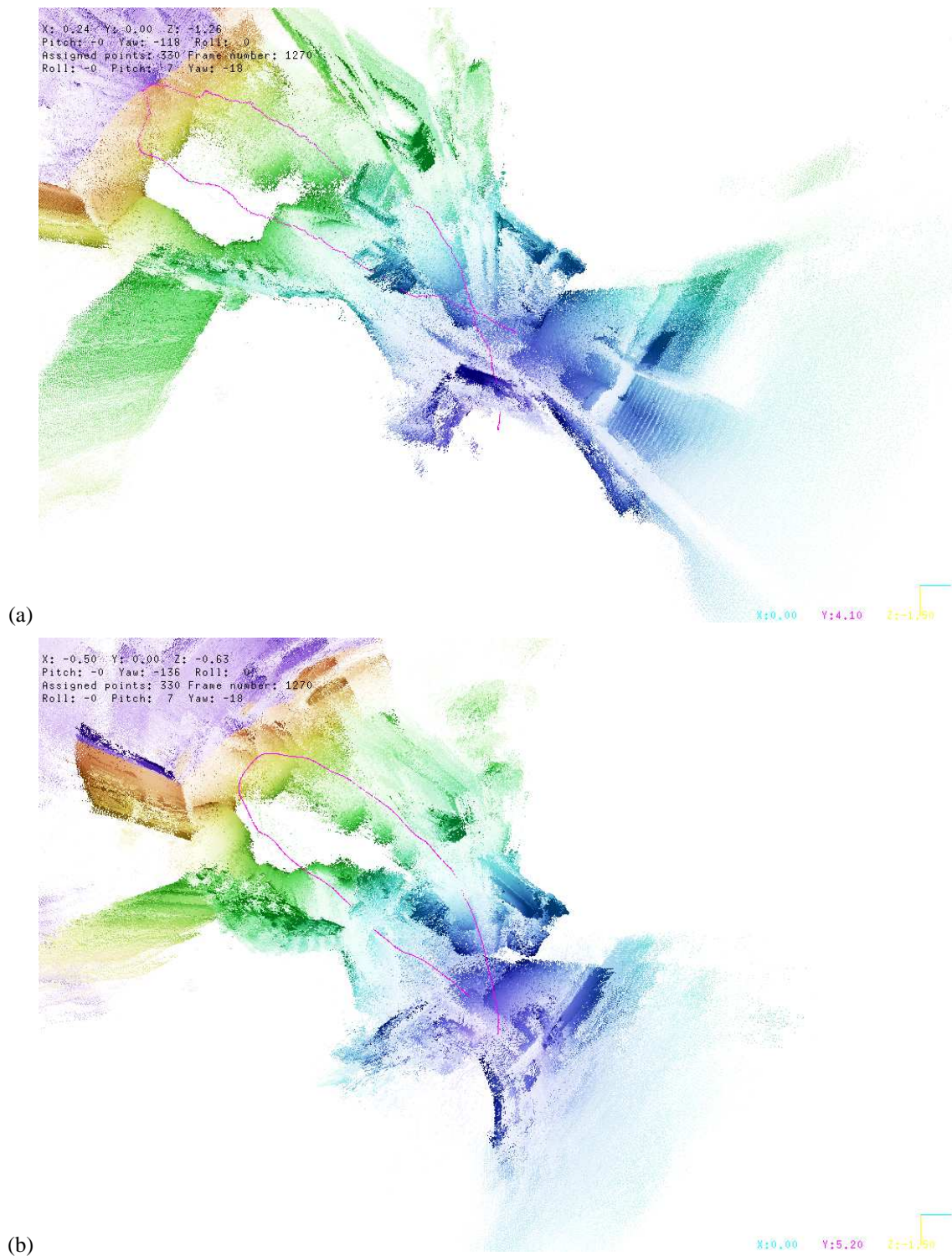
Fig. 10. (a) Top view of the resulting 3D map based on the estimated ego-motion. The map is squeezed at the end of the trajectory due to the error in the ego-motion estimate. (b) Improved map based on the fused ego-motion estimate.
