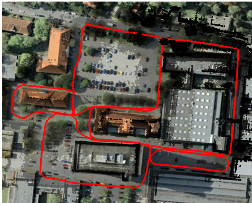
Fig. 11. Top: Comparison of the final combined result, applying LUM offline after processing the scans online with ELCH, against ground truth. Bottom: Image from Google Maps overlaid with the generated map (cf. Figure 2).
