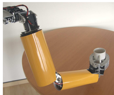
Fig. 3. 7 DOF human-scale anthropomorphic arm with 2 DOF gripper.
