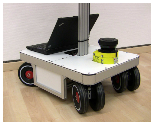
Fig. 2. Omnidirectional base with four individually steerable diff-drives.
