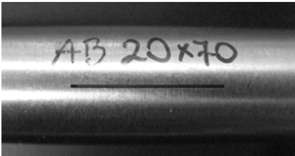
Figure 2. Defected tube before burst test
