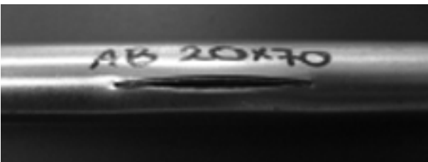
Figure 3. Defected tube after burst test
