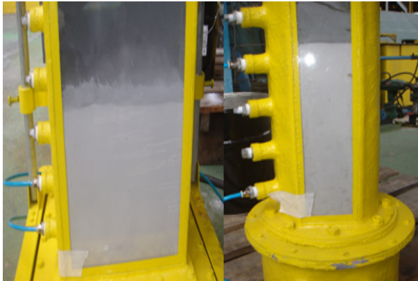
Figure 6. Permeameters used at Albras' laboratory to survey the minimum fluidization velocity of the powders used in the primary aluminum industry - source: (Vasconcelos, 2011) 10 .
