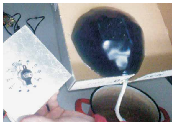
Figure 2. Ballistic gelatin with embedded heat source grid and external resistor selector.
