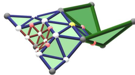
Figure 6: An example of a 3D mechanism. Different subdivision levels result in inflexible vertices (shown in red and yellow). Such vertices prevent folding of their support edge and therefore restrict the movability of the mechanism in regard to interactive displacement.
