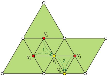
Figure 5: An example for propagation of inflexibility: 1. the two inflexible vertices  $v_1$  and  $v_2$  will cause  $v_a$  to become inflexible. 2.  $v_a$  together with the already existing inflexible vertex  $v_3$  induce a further inflexible point  $v_b$ .
