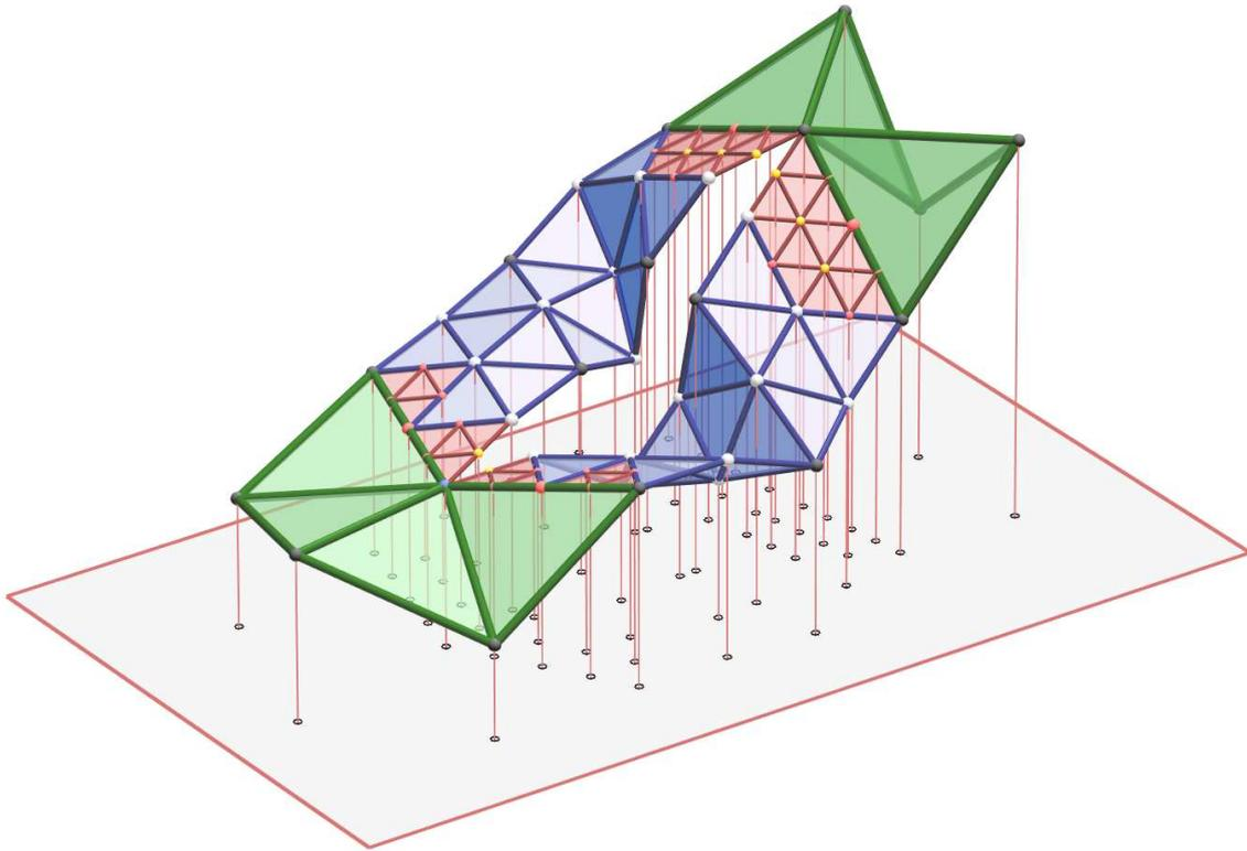
Figure 9: An example of a mesh with subdivisions up to level 2 which was designed with the described tool (level 0 = green, level 1 = blue and level 2 = red). Whereas triangles on subdivision level 0 and 1 have high flexibility, the level 2 triangles – as chosen in this example – have no further influence on the kinematic behavior of the mechanism. Inflexible vertices are shown in red and induced inflexible vertices are colored yellow.
