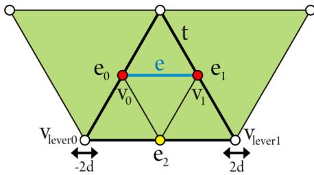
Figure 7: In order to keep the distance between two inflexible vertices  $v_0$  and  $v_1$  constant, their displacements have to be applied twice to the corresponding vertices  $v_{lever0}$  and  $v_{lever1}$  instead to  $v_0$  and  $v_1$ .
