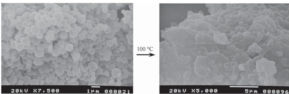
FIGURE 4 - Softening behaviour of PhOc02 as determined by SEM
