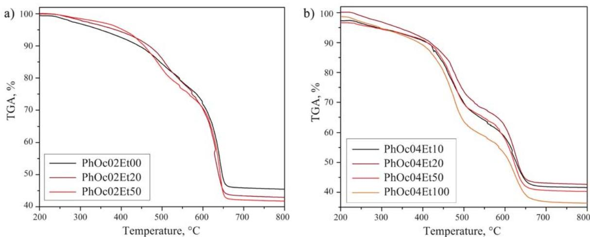
FIGURE 6 - Thermogravimetric curves for a) PhOc02 and b) PhOc04 polysilsesquioxanes
