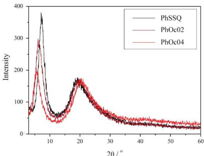
FIGURE 9 - XRD spectra of octyl-modified PhSSQ
