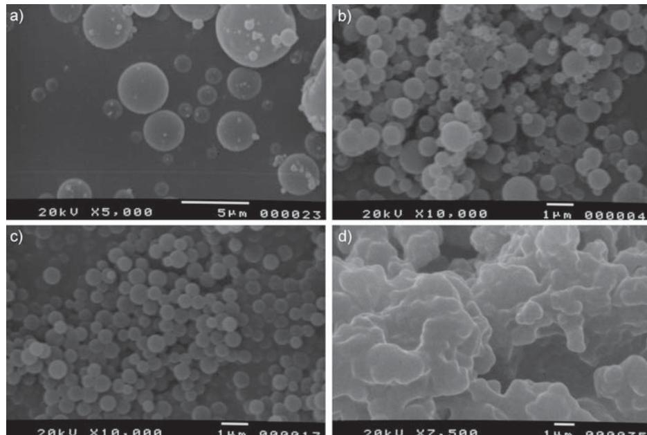
FIGURE 3 - Morphology of PhOc02 particles prepared with different quantities of ethanol: a) PhOc02Et00; b) PhOc02Et20; c) PhOc02Et50; d) PhOc02Et50 dispersed in water and ethanol
