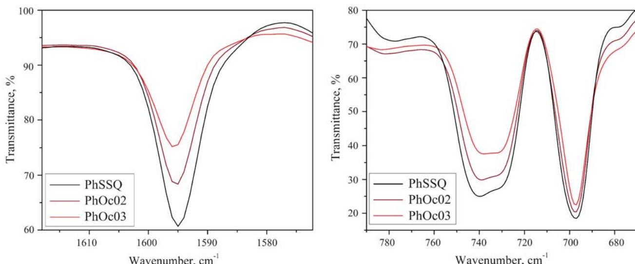
FIGURE 11 - Characteristic bands for semiquantitative analysis of octyl-modification of PhSSQs.
