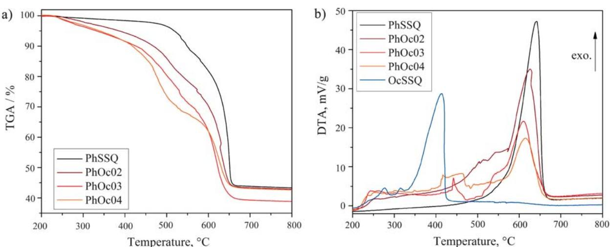
FIGURE 5 - Thermogravimetric (a) and DTA (b) curves for octyl-modified PhSSQs
