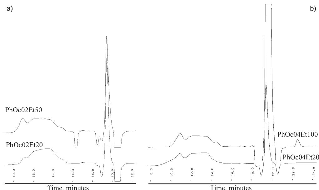
FIGURE 8 - GPC curves of a) PhOc02 and b) PhOc04 polysilsesquioxanes
