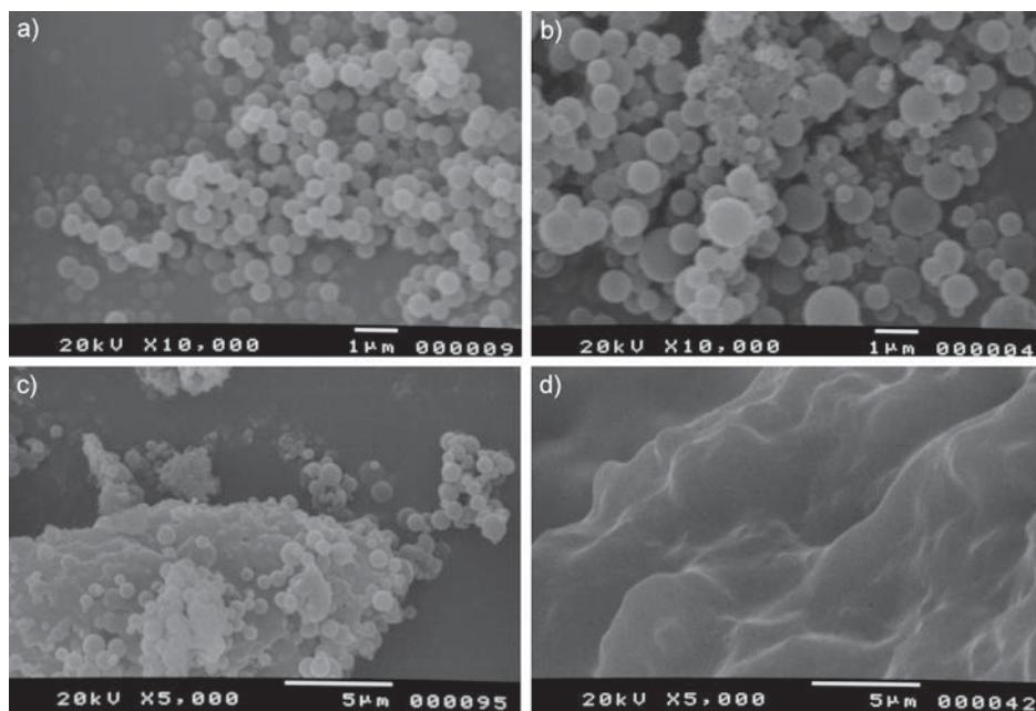
FIGURE 2 - Morphology of alkyl-modified polysilsesquioxanes: a) Ph-SSQ; b) PhOc02; c) PhOc03; d) PhOc04
