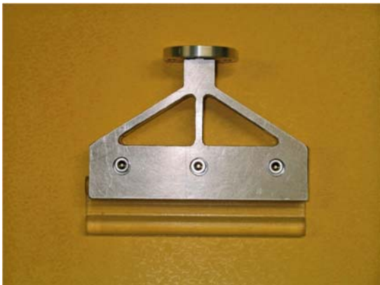
FIGURE 5 – Pure shear specimen for elastomer fatigue tests
