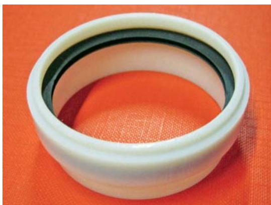
FIGURE 6 – Two components rapid prototyping of an integrated pipe sealing
