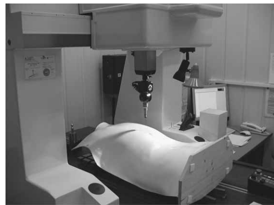
Fig. 3. A mechanical tactile coordinate device, DEA Iota Diamond measures a plastic model.
