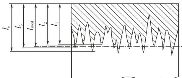
Figure 1 Determination of boride layer thickness [5]
