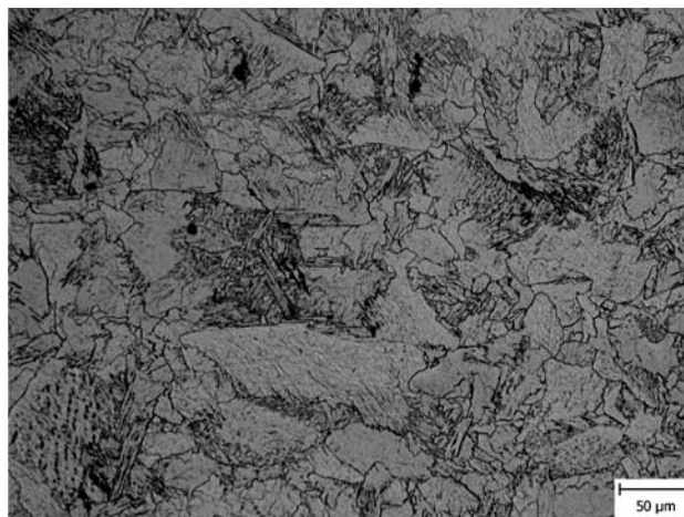
Figure 6 Microstructure of weld metal of specimen from non-treated sheet
