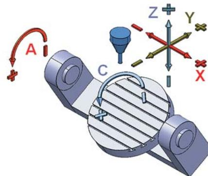
Figure 1 5D machine structure with swivel rotary table
