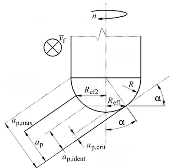
Figure 6 Longitudinal downward milling
