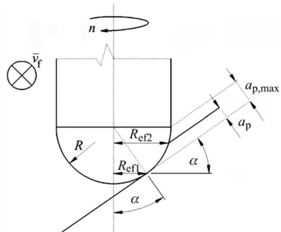
Figure 5 Longitudinal upward milling
