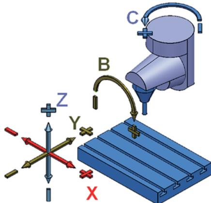
Figure 2 5D machine structure with tool rotation in two axes
