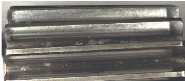
Figure 8: Worn locomotive pinion
