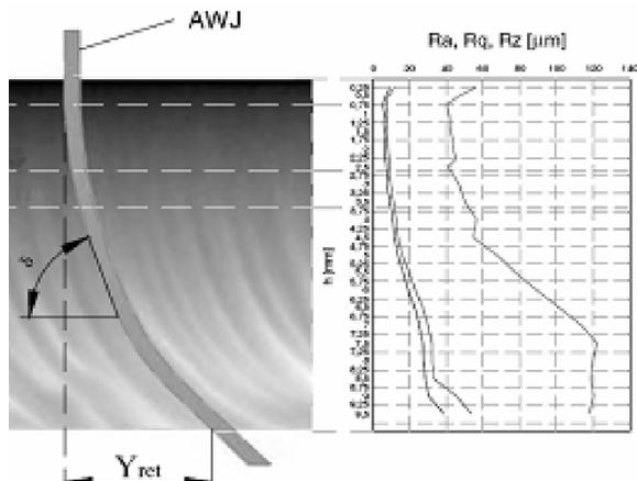
Figure 6. Change of surface roughness, depending on the depth of cutting [4]
