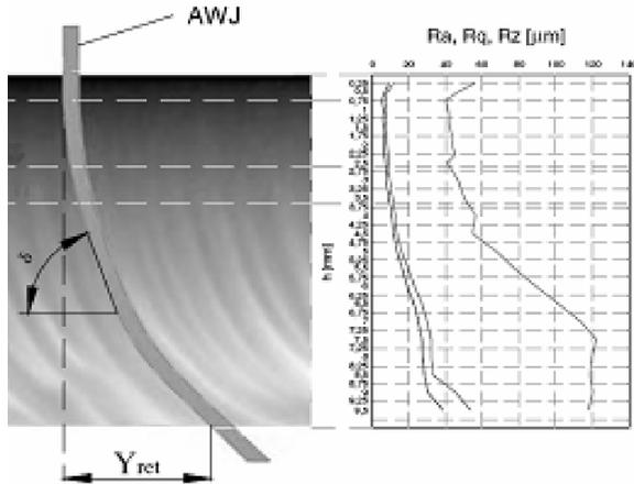
**Figure 6.** Change of surface roughness, depending on the depth of cutting [4]
