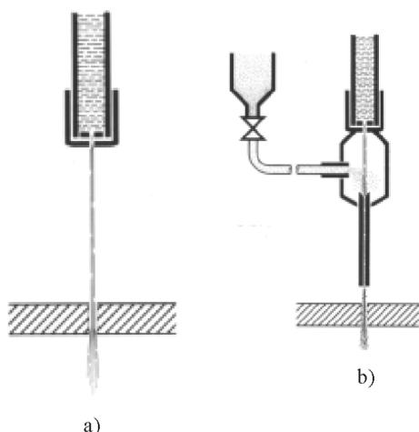
**Figure 1.** Scheme of the processing without abrasive water-jet a) and with abrasive water-jet b)
