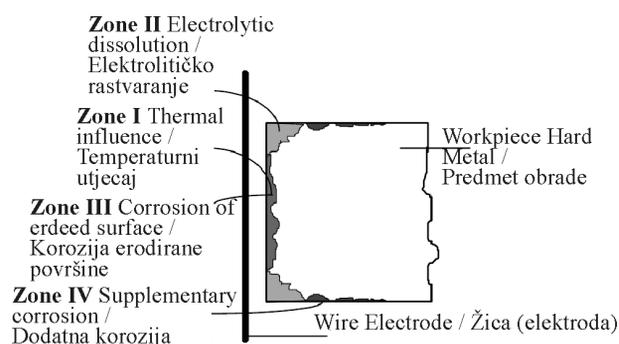
**Figure 2.** Characteristic zones on the hard metal machined surface [2]
