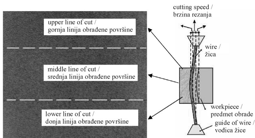
Figure 7. Surface appearance machined with wire electrical discharge machining [7]
