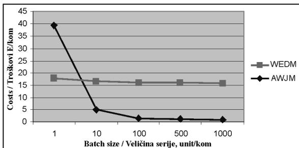
**Figure 13.** Dependence on manufacturing cost per unit of the batch size for the machining by abrasive waterjet (AWJ) and for the wire electrical discharge machining (WEDM)
