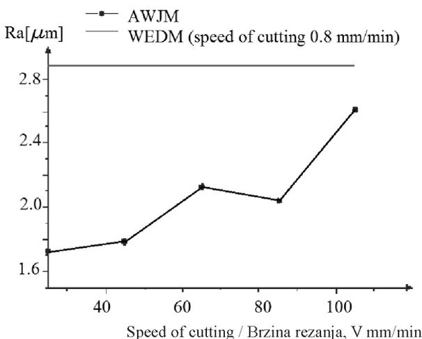
**Figure 12.** Comparative review of depending value Ra of cutting speed with the wire electrical discharge machining and machining by abrasive waterjet
