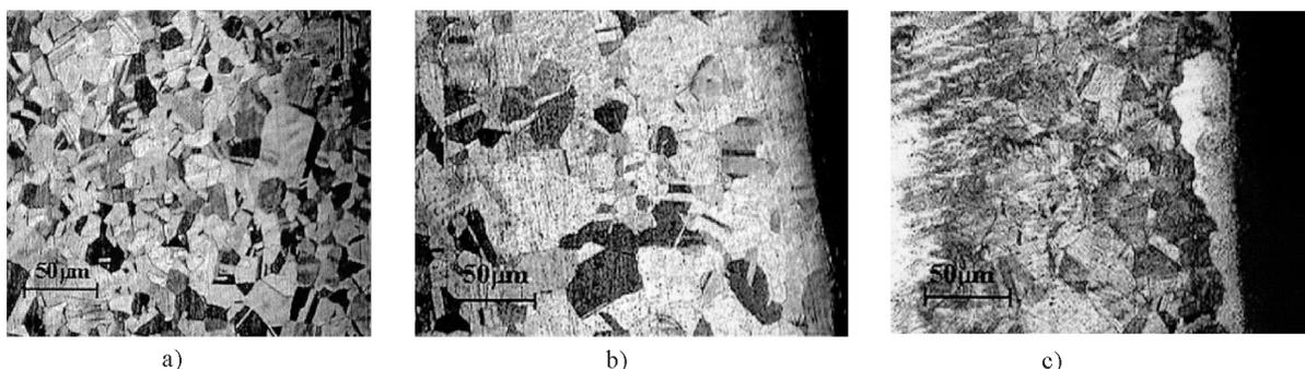
Figure 8. The microstructure of steel C 4580 without the machining (a), after the machining by abrasive waterjet (b) and after wire electrical discharge machining (c) [1]
