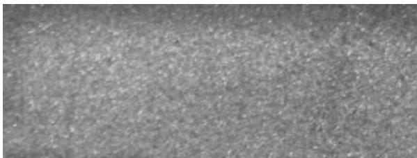
**Figure 3.** Surface machined with abrasive water-jet
