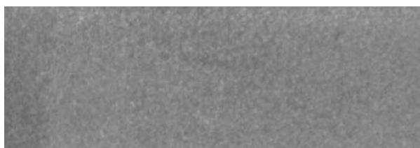
**Figure 4.** Surface machined with electrical-discharge machining
