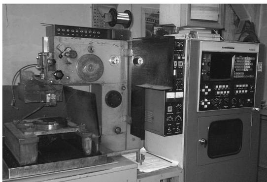
Figure 10. Spark erosion machine ANUC TAPE CUT-MODEL H
