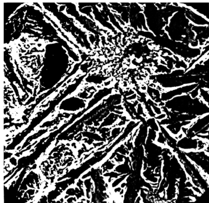
Figure 6. Fracture surface in jaw arm surface area, 1000:1
