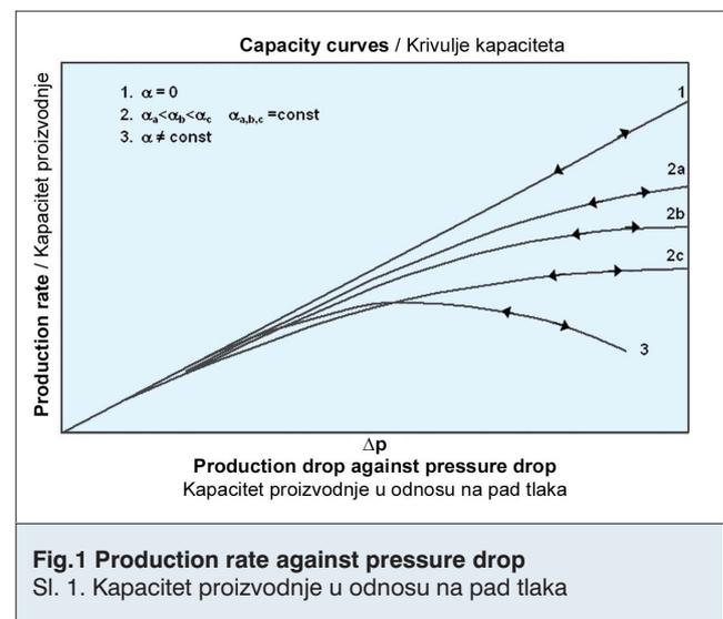
Fig.1 Production rate against pressure drop
