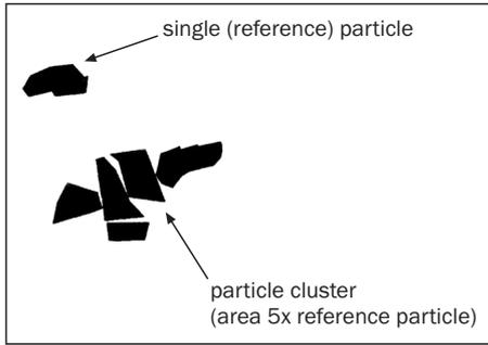
Figure 7 - Evaluation of the projected images for quantifying of particle clusters by image analysing computer
