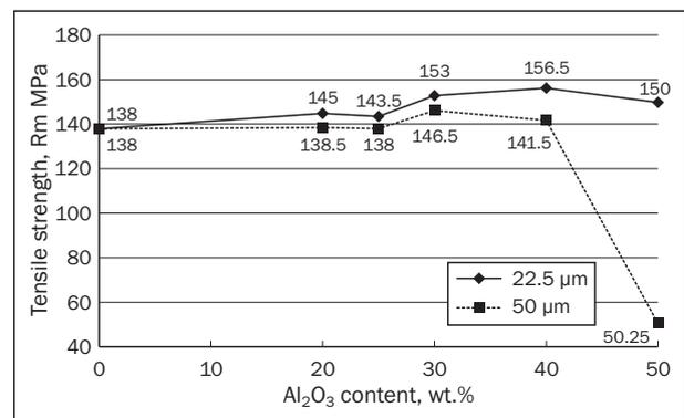
Figure 10 - Tensile strength of the  $Al/Al_2O_3$  composites as a function of the content and particle size of  $Al_2O_3$ (Zesk)
