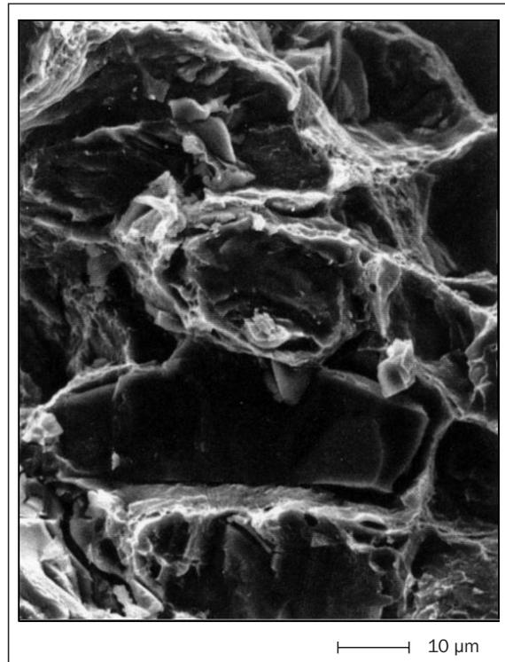
Figure 18 - Al+40wt%Al<sub>2</sub>O<sub>3</sub>(50µm)
