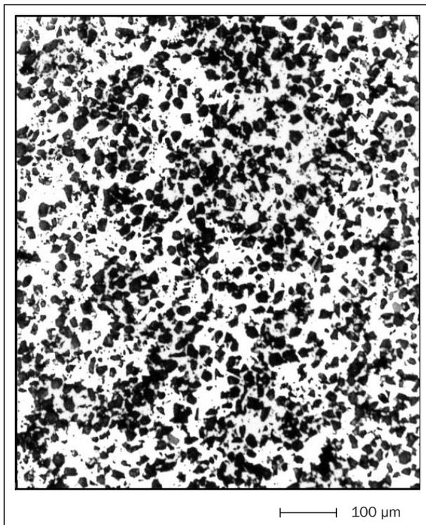
Figure 5 - Al+50wt%Al<sub>2</sub>O<sub>3</sub>(22.5µm)
