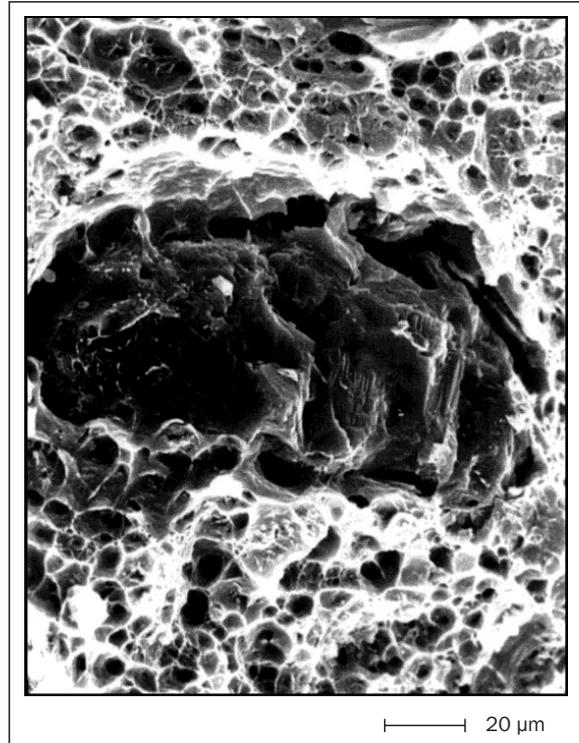
Figure 16 - Al+20wt%Al<sub>2</sub>O<sub>3</sub>(50µm)
