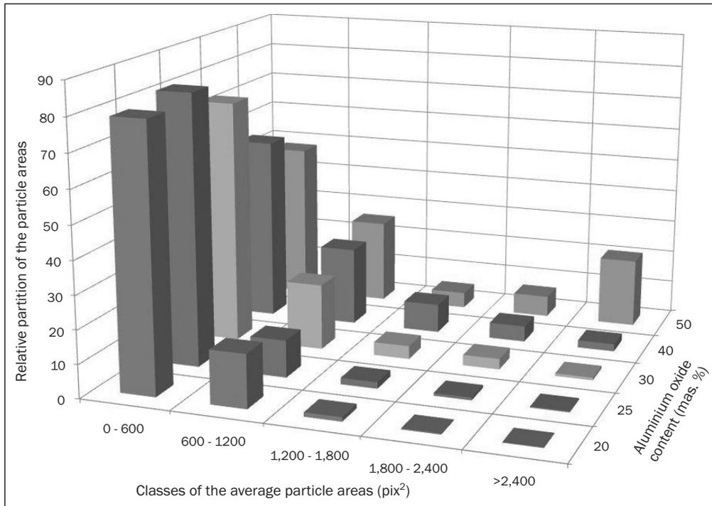
Figure 8 - Distribution of the average particle areas for different  $Al_2O_3$  particle contents: Standard particle area was  $100-600\text{pix}^2$
