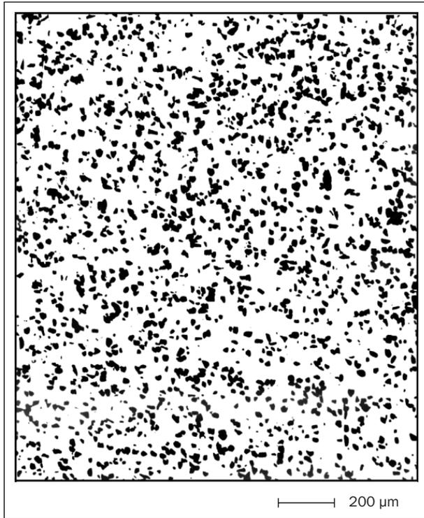
Figure 3 - Al+20wt%Al<sub>2</sub>O<sub>3</sub>(22.5µm)
