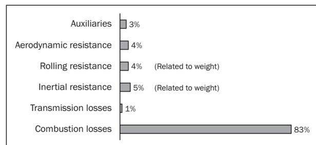
Figure 2 - Driving force for weight reduction - complete energy flow in EU combined (5-cyl-gasoline engine) [2][15]
