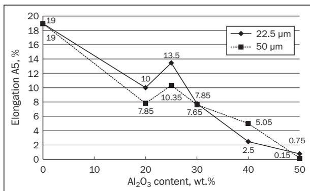
Figure 13 - Elongation of Al/Al<sub>2</sub>O<sub>3</sub> composites as a function of the content and particle size of Al<sub>2</sub>O<sub>3</sub>(Zesk)
