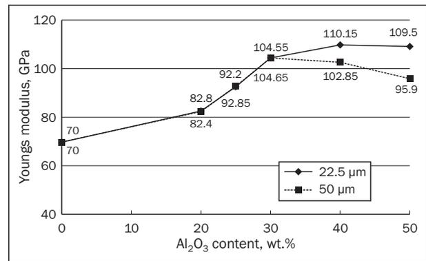
Figure 12 - Young's modulus of Al/Al<sub>2</sub>O<sub>3</sub> composites as a function of the content and particle size of Al<sub>2</sub>O<sub>3</sub>(Zesk)
