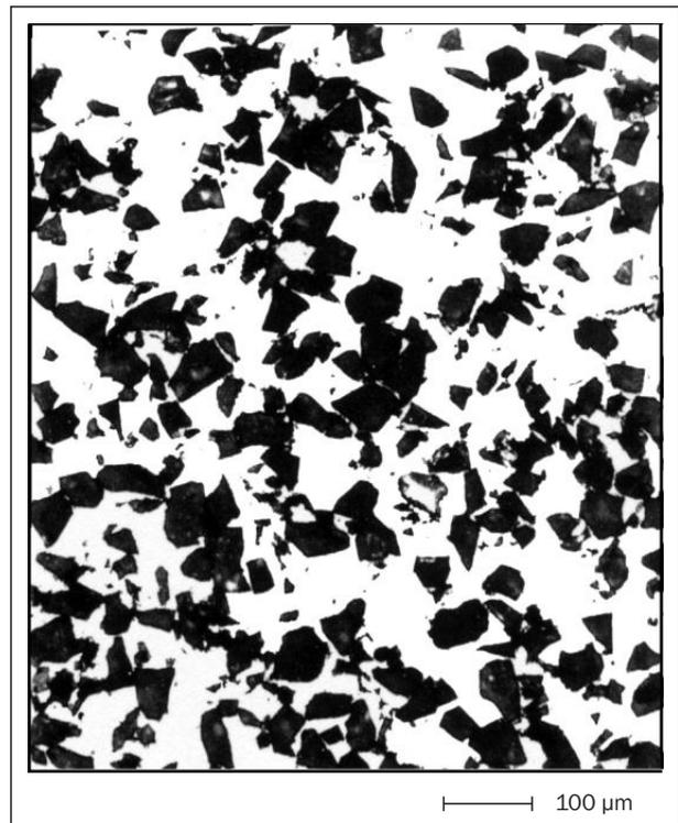
Figure 6 - Al+50wt%Al<sub>2</sub>O<sub>3</sub>(50µm)
