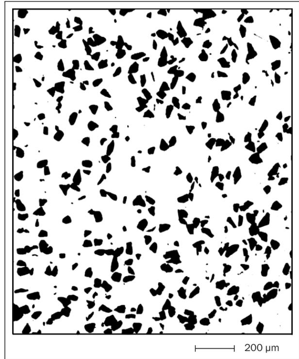
Figure 4 - Al+20wt%Al<sub>2</sub>O<sub>3</sub>(50µm)
