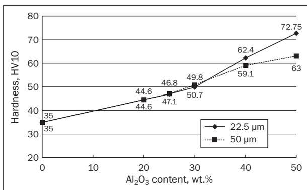
Figure 9 - Hardness of the  $Al/Al_2O_3$  composites as a function of the content and particle size of  $Al_2O_3$ (Zesk)
