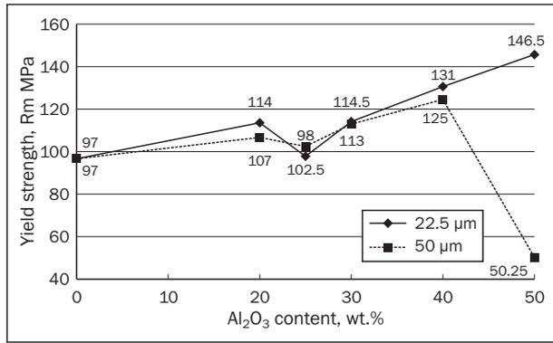
Figure 11 - Yield strength of the Al/Al<sub>2</sub>O<sub>3</sub> composites as a function of the content and particle size of Al<sub>2</sub>O<sub>3</sub>(Zesk)
