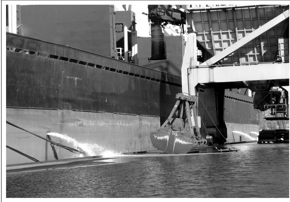
Figure 1 - Discharge of ballast water above the level of the pier from the upper side wing tanks of a bulk-carrier
