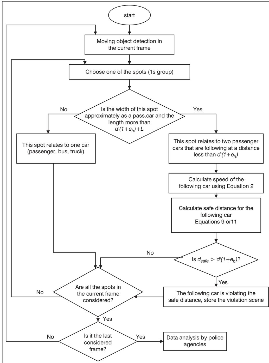
Figure 9 - Algorithm for detecting safe distance violation
