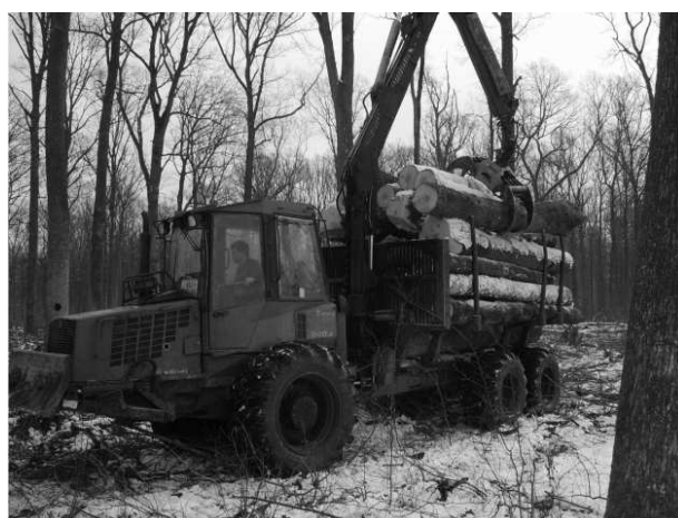
Slika 4. Istraživani forvarder Valmet 840.2 u radu Fig. 4 Researched forwarder Valmet 840.2
