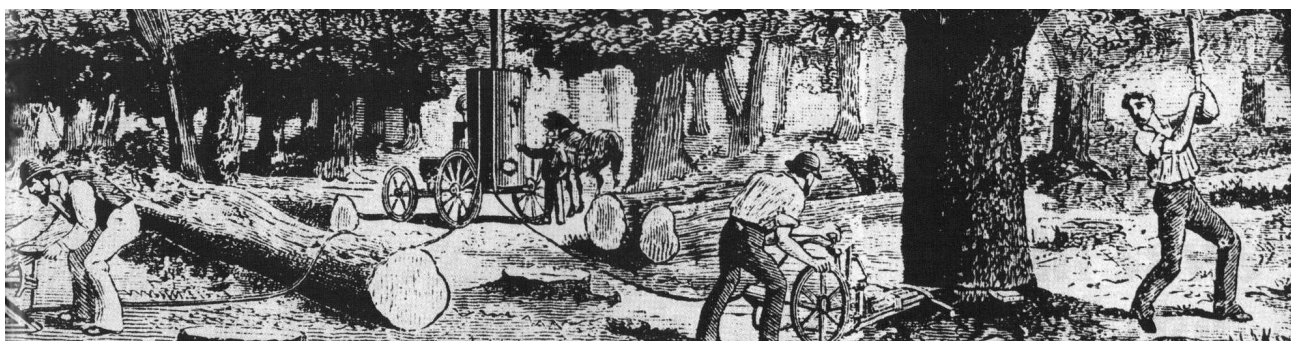
Slika 4. Ransomova parna pila Fig. 4 Ransome's steam powered saw
