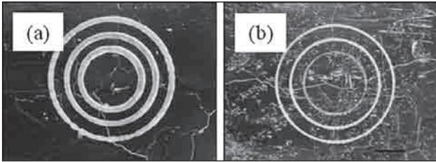
**Figure 4** Macrostructure of alloys M1 (a) and M2 (b) with visible tracks left by ball during the ball-on-disc abrasive wear test. 12 x
