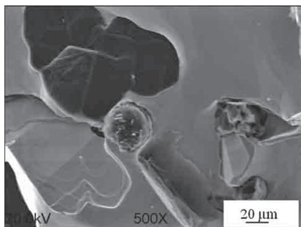
**Figure 3** SE image of the fracture of alloy M2 containing 1,25 wt. % C with visible precipitates of lamellar and spheroidal graphite
