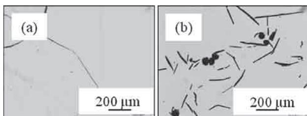
**Figure 2** Microstructure of alloy M1 containing 0,2 wt. % C (a) and alloy M2 containing 1,25 wt. % C (b). Image obtained under light microscope
