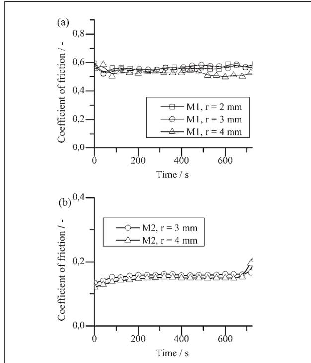
**Figure 6** The coefficient of friction determined for alloys M1 (a) and M2 (b).
