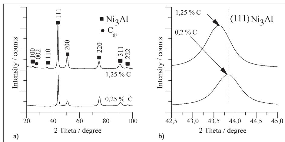
**Figure 1** Comparative X-ray diffraction patterns of alloys M1 and M2 containing 0,2 % (a) and 1,25 % (b), respectively
