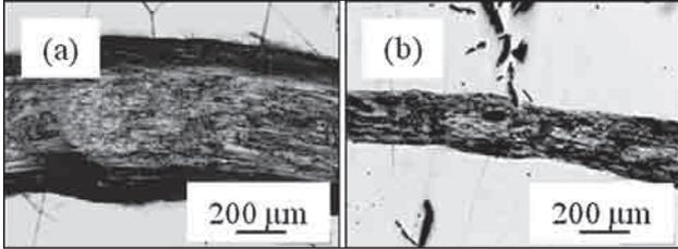
**Figure 5** Macrostructure of alloys 0,2 wt. % C (a) and 1,25 wt. % C (b) with visible tracks left by ball during the ball-on-disc abrasive wear test
