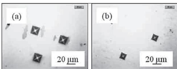
**Figure 8** Microstructure of alloys M1 (a) and M2 (b) with visible MHV indentation marks
