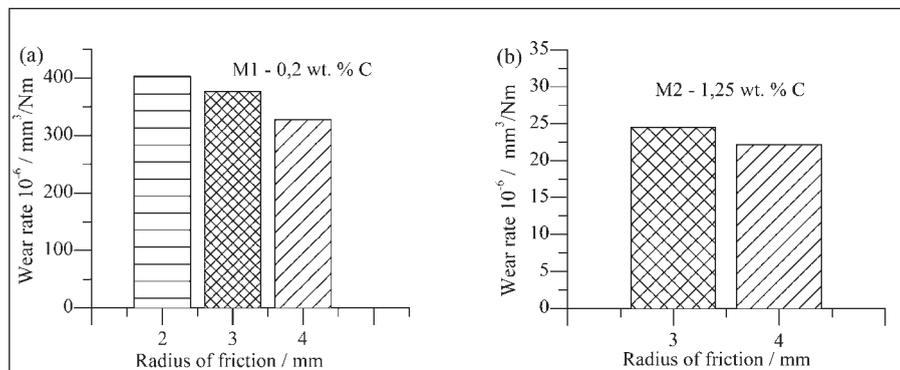
**Figure 7** Wear rate under different friction radii determined for alloys M1 (a) and M2 (b)
